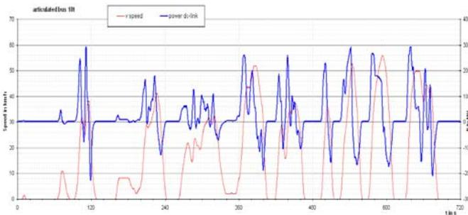
Figure 2: Line 53 power demand from GPS measuring during the first 12 minutes
