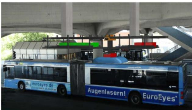
Figure 9: Picture of Battery change system integrated in bus terminal "Aidenbachstr."
