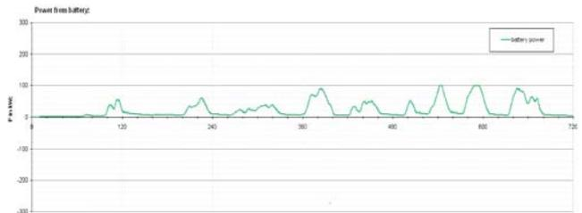
Figure 4: line 53 power from battery **with** support of ultra capacitors during the first 12 minutes
