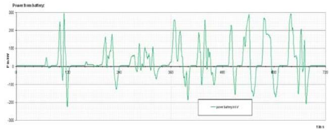
Figure 3: line 53 power from battery **without** ultra capacitors during the first 12 minutes
